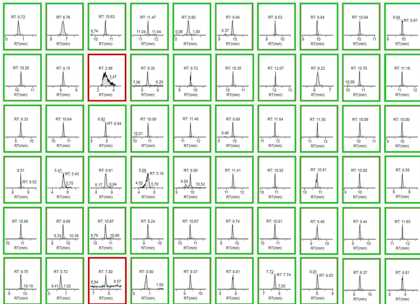
Figure 6. Randomly chosen parent ion peaks in tea matrix at 5 ng/g concentration level. Compounds from top left to right bottom: Acephate, acetamiprid, chloroxuron, clofentezin, aminocarb, azaconazole, isocarbophos, diethofencarb, trietazin, azinphos-me, ethiofencarb, bromacyl, carbendazim, carbofuran, chlorantraniliprole, mepronil, etoxazole, chloridazon, dimetamethrin, cyflufenamide, flutriafol, triazophos, fenthion-sulfoxide, diflubenzuron, trifloxystrobin, flazasulfuron, tralkoxydim, benfuracarb, propazine, ethofumesate, dithiopyr, desmethyl-primidicarb, desmethryn, flumetsulam, bensulfuron-me, prosulfocarb, tebufenozide, carfentrazone-et, esprocarb, hexazinone, neburon, diuron, piperonyl-butoxide, sulfotep, triticonazole, buprofezin, cyazofamide, bitertanol, benzoximate, hexaflumuron, forchlorfenuron, cyromazine, metholcarb, methomyl, metabromuron, metosulam, metoxuron, metribuzin, metazachlor, and piperophos. Compounds marked with red refer to asymmetry factor > 1.5 for carbendazim and missing fragment ion ratio for metholcarb at concentration level close to IDL.
